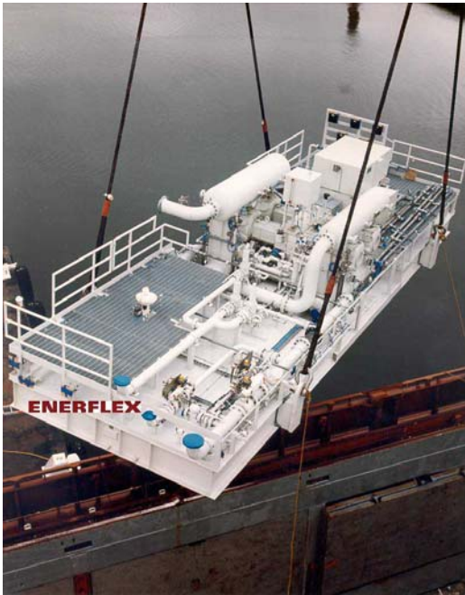
Figure 10. A large reciprocating compressor for NG service; 3,000 hp electric motor drive.
