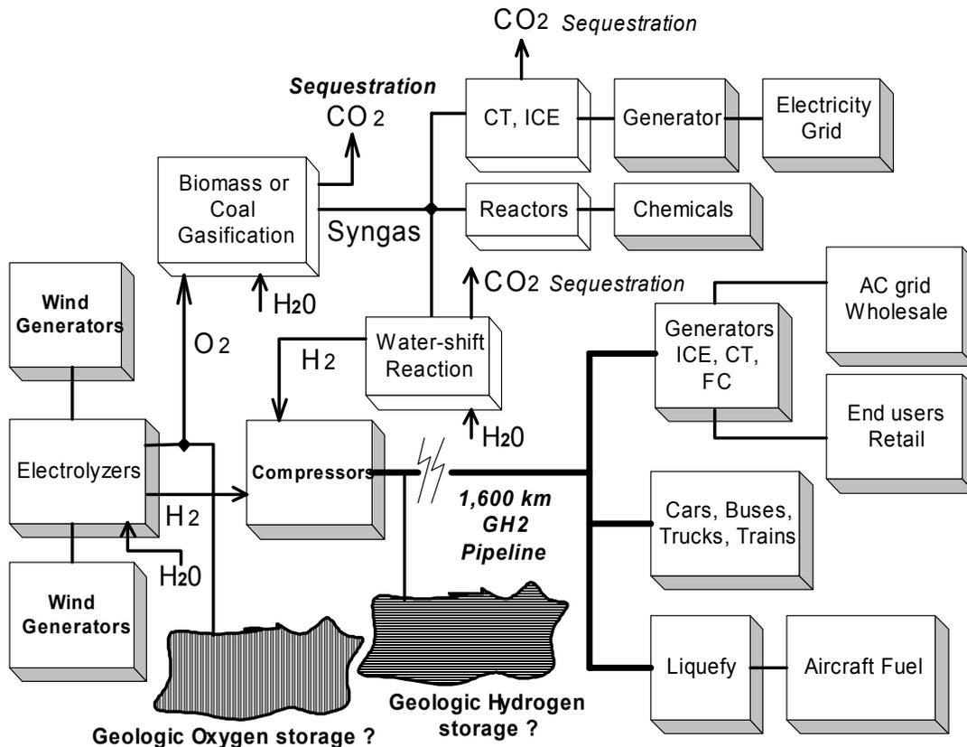
**Figure 4.** Synergy with biomass gasification or “zero emissions” coal gasification plants adjacent to wind energy sources, using byproduct oxygen from electrolyzers for oxygen-blown gasification. Large-scale geologic storage feasibility of hydrogen and oxygen is unknown.
