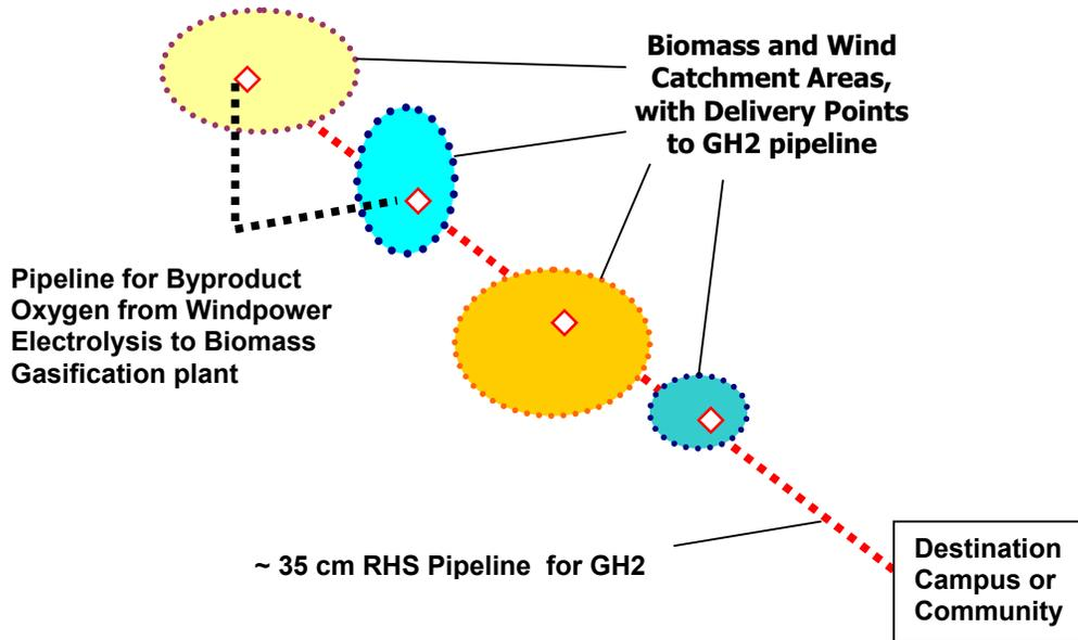
**Figure 9.** International Hydrogen Transmission Test Facility (IHTTF) concept: a corridor of distributed collection from distributed generation. RHS pipeline ~ 50-100 km long, ~ 10-100 MW , ~ 35 cm diam.
