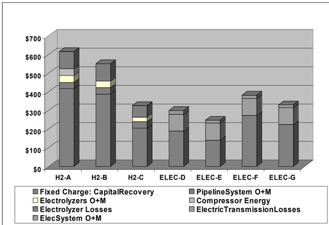
**Figure 5.** Annual Transmission Costs and Energy Losses, \$US 2001 millions. 4 GW (nameplate) windplant, 1600 km transmission from North Dakota to Chicago. “H2- “ are hydrogen pipeline cases; “ELEC- “ are HVDC electric transmission cases [3].
