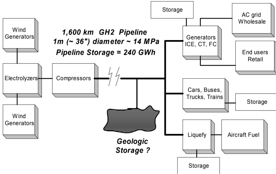
**Figure 2.** “Renewables Hydrogen Service” (RHS) pipeline Transmission, delivering GH<sub>2</sub> from distant wind resources to various users, with potential storage schemes in addition to pipeline storage.
