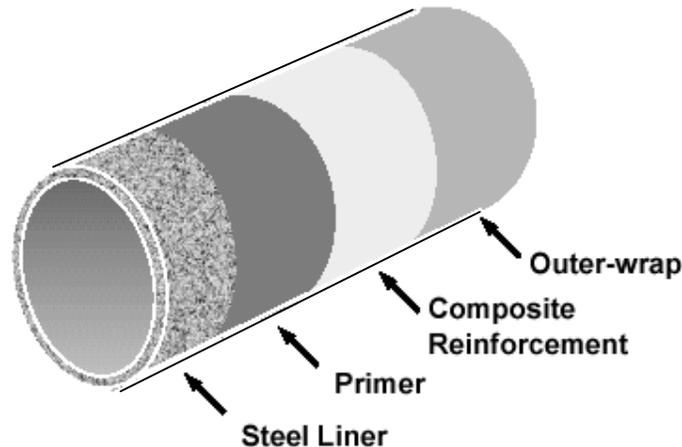
**Figure 3.** Composite Reinforced Line Pipe (CRLP™).
