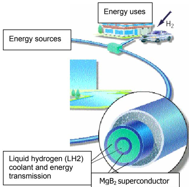
**Figure 8.** Superconducting low voltage direct current (LVDC-SC) “Energy Pipeline” proposed by Electric Power Research Institute (EPRI) [45]. Estimated 100 GW electrical plus 100 GW liquid hydrogen power transmission capacity. Magnesium diboride (MgB<sub>2</sub>) superconductor.
