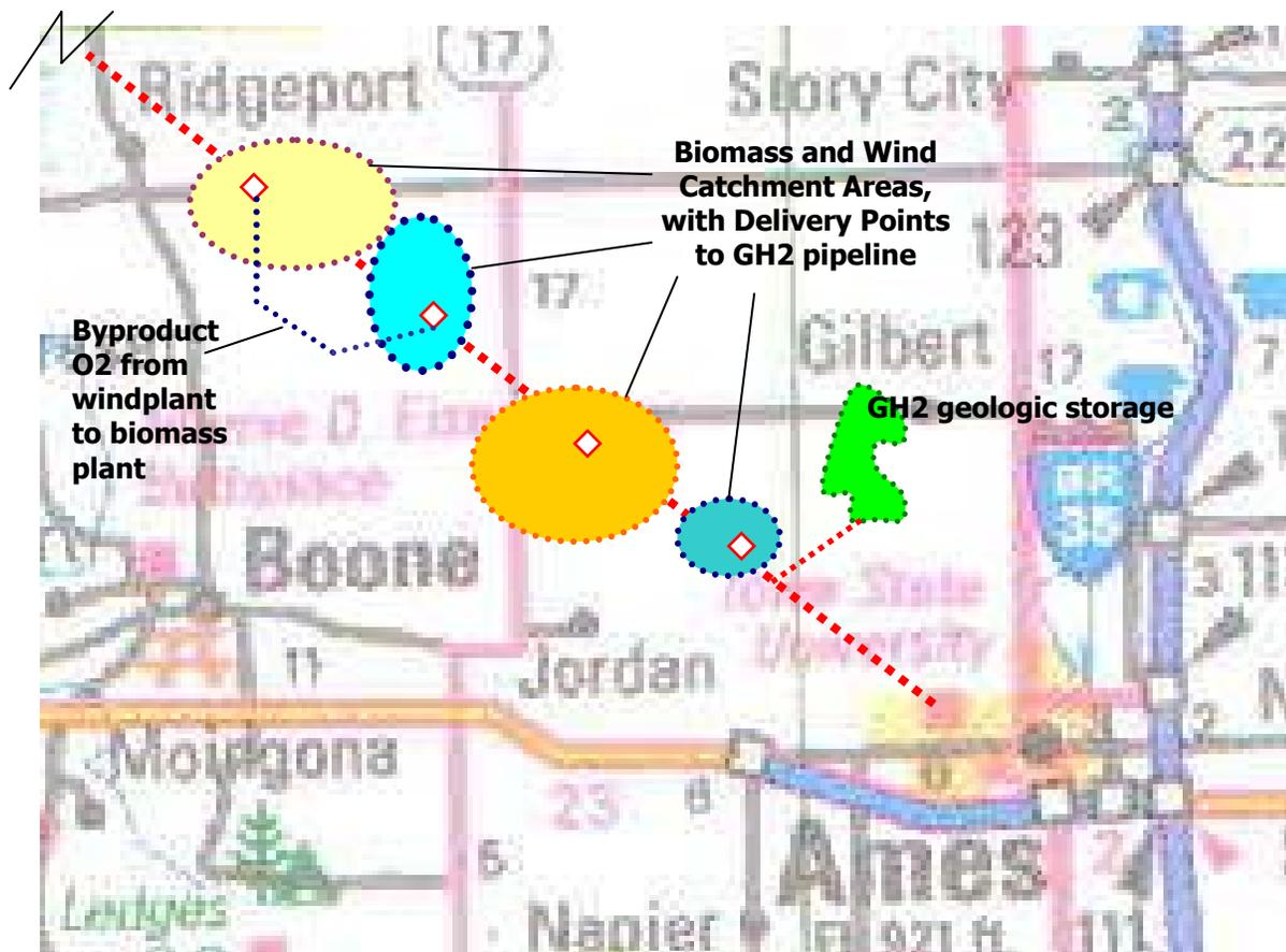
**Figure 6.** Detail of “Distributed Collection” (DC): GH2 gathering topology as a continuous collection and transmission corridor, rather than a transmission line. The economic gathering radius varies with each resource. Byproduct O<sub>2</sub> from wind-to-hydrogen electrolysis is supplied to adjacent biomass gasification plants producing GH<sub>2</sub> for the pipeline.
