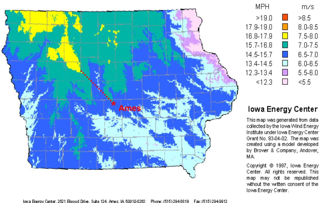
**Figure 5.** Candidate location for the IHTDF. Approximately 60 miles (100 km) GH2 pipeline from the windy region west of Ft. Dodge, Iowa, to Iowa State University and USDOE Ames Laboratory at Ames, Iowa.
