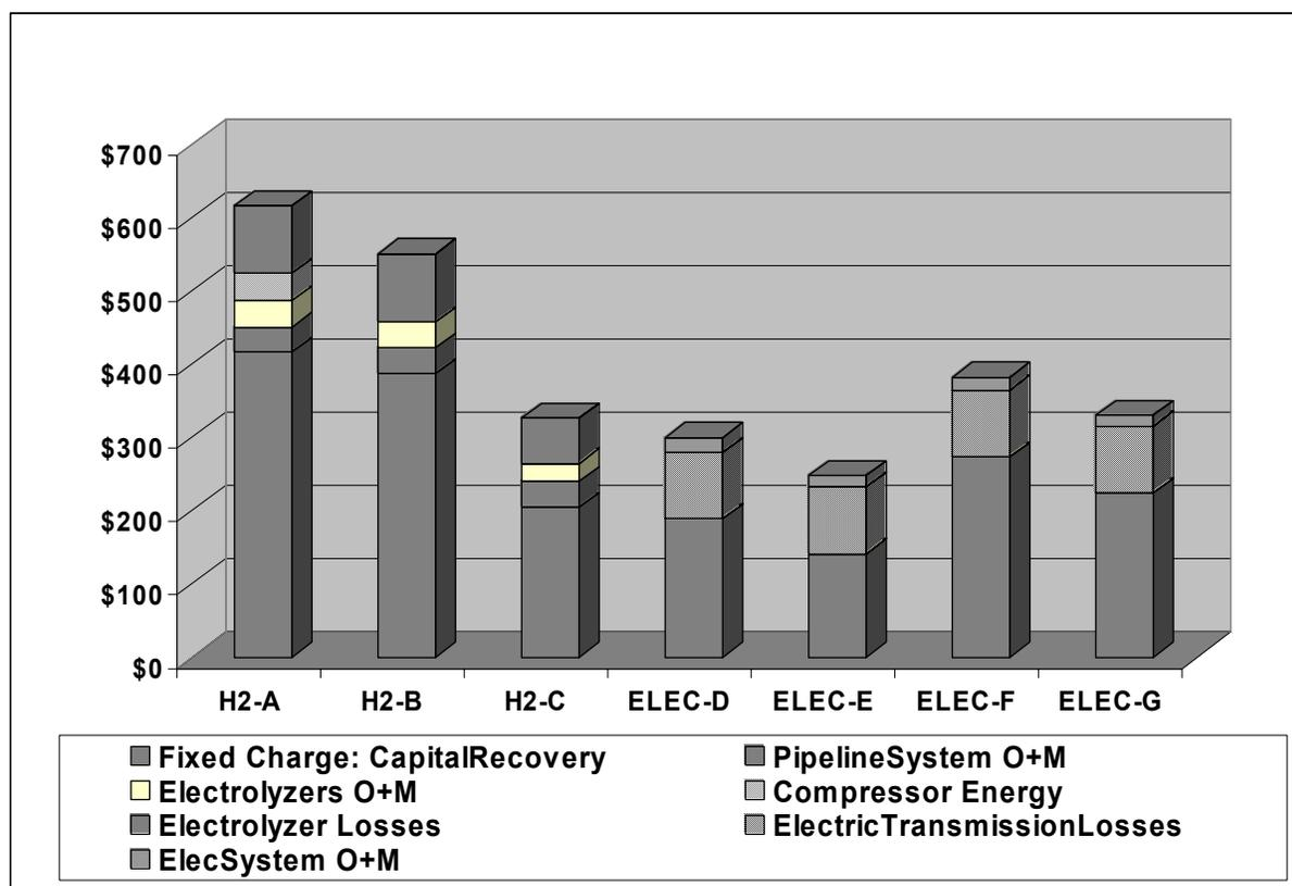
**Figure 2.** Annual Transmission Costs and Energy Losses, \$US 2001 millions, for a 4 GW (nameplate) windplant, 1600 km transmission from North Dakota to Chicago. “H2- “ are hydrogen pipeline cases; “ELEC- “ are HVDC electric transmission cases
