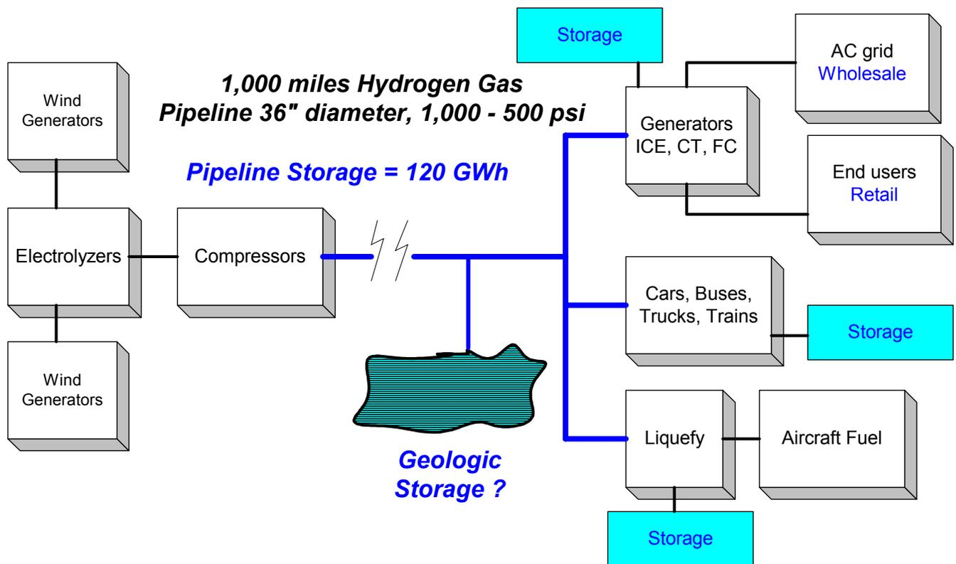
**FIGURE 1.** Hydrogen transmission with pipeline storage and diverse users of hydrogen fuel. Pipeline, alone, stores 120 GWh. Prospects for large-scale geologic storage in Great Plains are unknown, but could make wind energy “dispatchable”.
