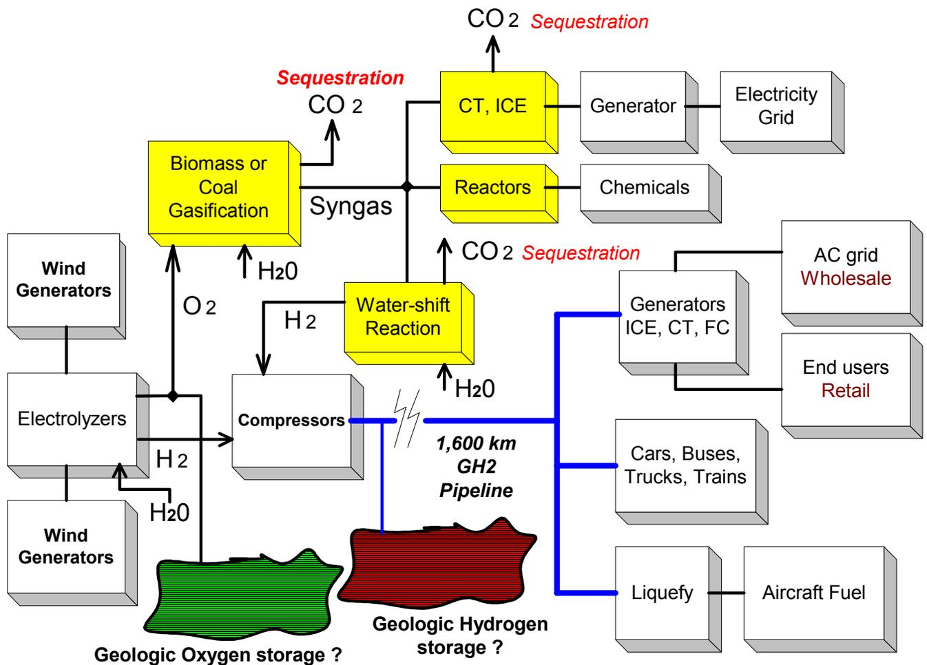
**Figure 3.** “Renewables Hydrogen Service” (RHS) pipeline transmission, delivering GH<sub>2</sub> from distant wind resources to various users, with potential storage schemes in addition to pipeline storage. Synergy with biomass gasification or “zero emissions” coal gasification plants adjacent to wind energy sources, using byproduct oxygen from electrolyzers for oxygen-blown gasification. Large-scale geologic storage feasibility of hydrogen and oxygen is unknown.
