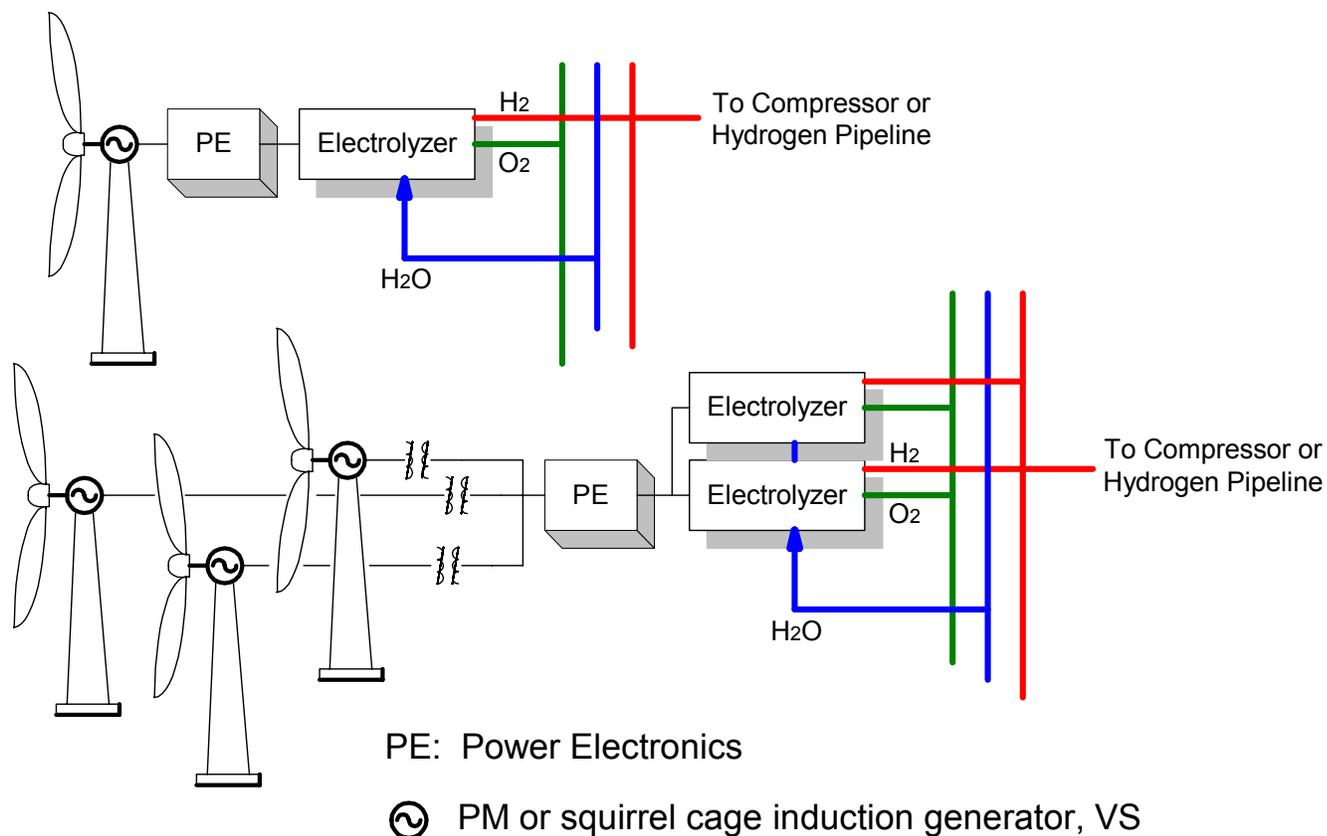
**Figure 4.** Wind generators driving only direct current (DC) electrolyzers, may simplify and lower the cost of power electronics. Variable speed (VS) permanent magnet (PM) or low-cost induction generators may be used, to further lower system capital and O&M costs.
