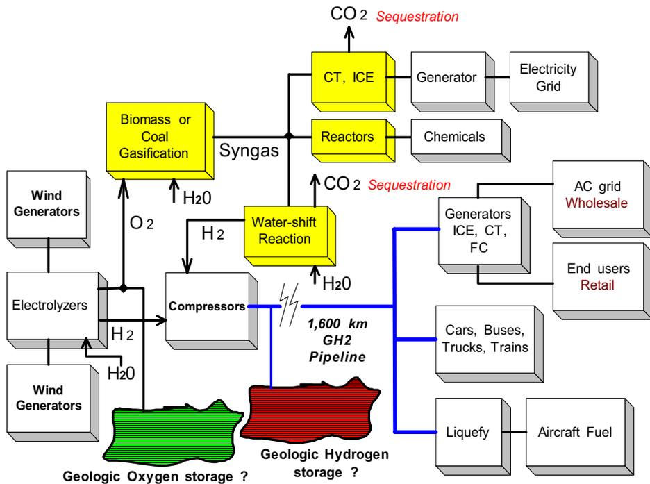
Figure 5. IRHTDF advanced system with potential biomass and “near zero emissions” biomass or coal gasification synergy, using oxygen (O<sub>2</sub>) byproduct of electrolysis. Feasibility of large-scale geologic storage of H<sub>2</sub> and O<sub>2</sub> in the USA Great Plains is unknown.
