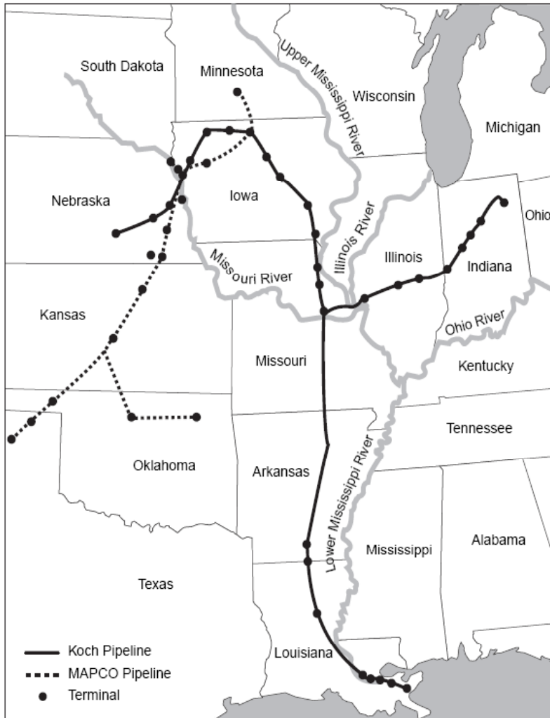
Figure 9. Existing NH 3 pipelines and storage terminals. Storage is in refrigerated, liquid, above-ground steel tanks of 10 – 60,000 tons each.
