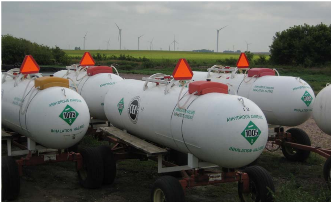
Figure 8. Clipper Windpower 2.5 MW turbines in background with liquid anhydrous ammonia ( \text{NH}_3 ) nitrogen fertilizer “nurse tanks”, \sim 5 \text{ m}^3 each. Wind-generated electricity can be locally converted to \text{NH}_3 for fertilizer and fuel, without expansion of the electricity transmission grid. September '07, NE Iowa.
