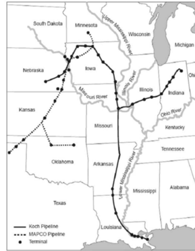
Fig. 13. Extant liquid NH 3 pipeline and storage terminal network, handling ~15 MMT per year, primarily for N-fertilizer, of which ~60% is imported.
