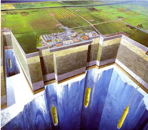
Fig. 6. Multiple large, solution-mined salt caverns in “domal” salt, suitable for high-pressure storage of GH2. A typical cavern will store 90,000 MWh as 2,500 net MT of GH2 at 70-150 bar in ~800,000 cubic meters physical volume. Total capital cost of cavern, GH2 cushion gas, and shared surface facility is ~ $ 15M; ~$ 0.20 / kWh
