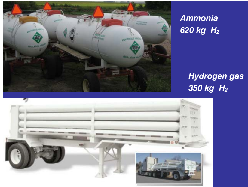
Figure 2. Energy storage: (above) Agricultural fertilizer liquid NH 3 “nurse tank”: capacity 1,450 gallons @ 265 psi = 620 kg hydrogen. Capital cost $9.5K (below) Gaseous hydrogen tube trailer: capacity 5,800 gallons @ 3,200 psi = 350 kg hydrogen. Capital cost $750K
